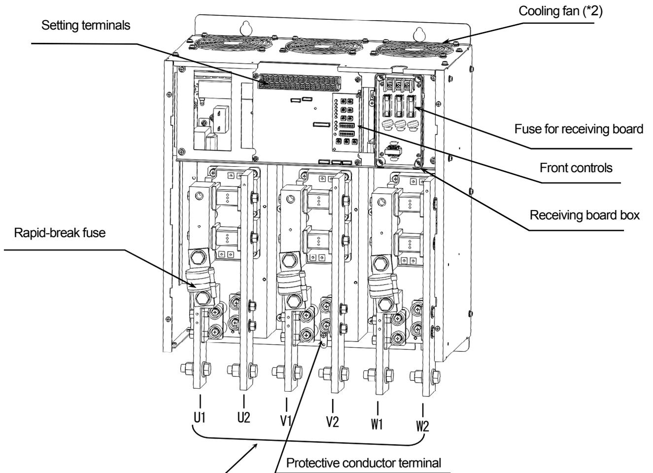
(\*2) For units with rated currents of 300A, 2 cooling fans are provided.
