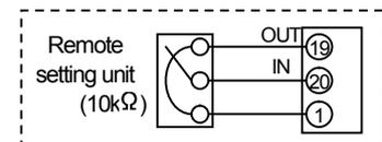
The final slope setting value is the product of the slope setting (Slope A) set by either [Front panel setting (SET1 trimmer)] or [Remote setting input (AI1)] and [Slope using the control input signal (Slope B)].
