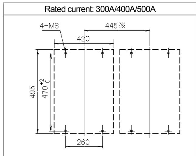
※ Caution: Minimum distance when plural instruments are installed side by side
