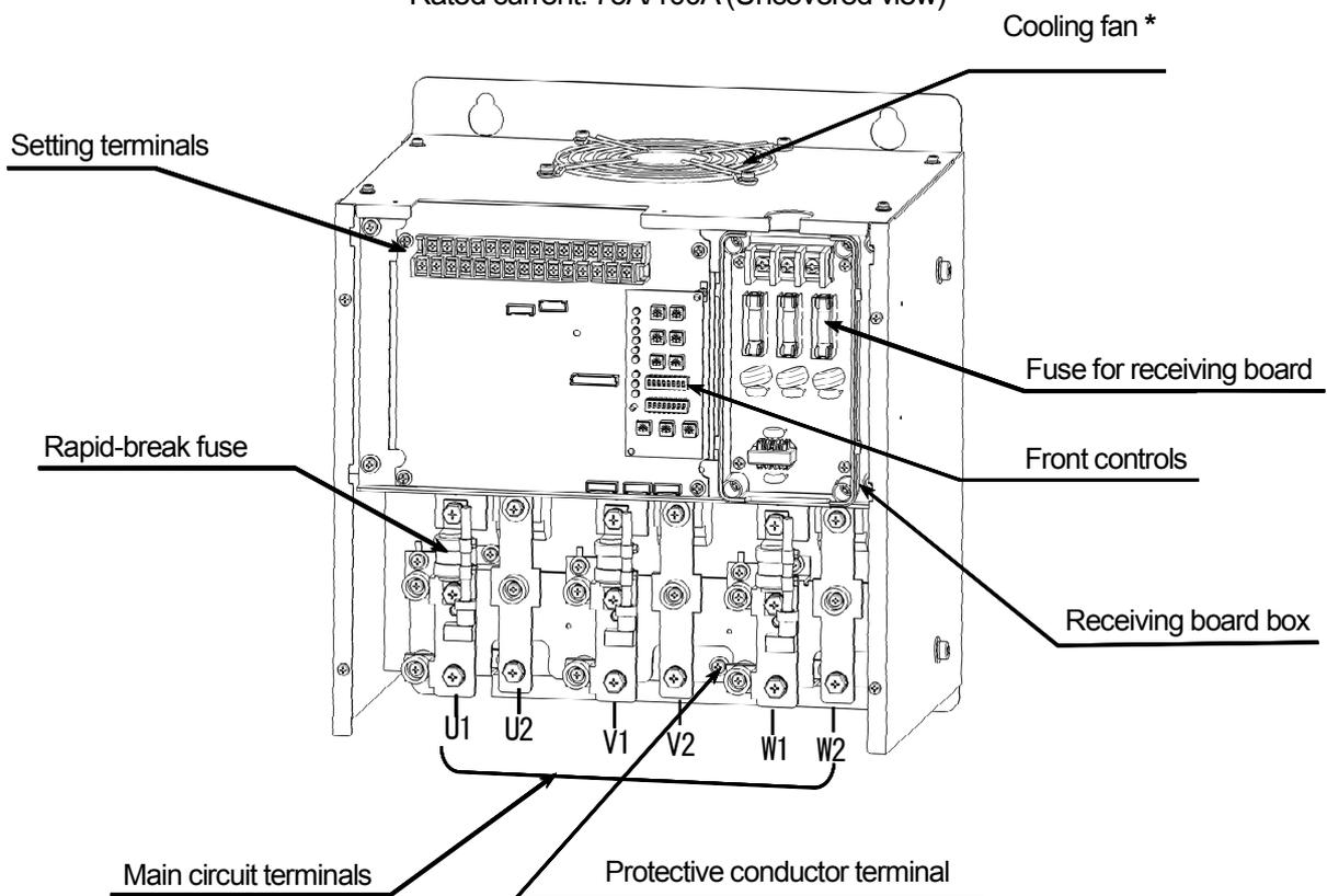
\* Cooling fans not mounted for a rated current of 75A units
