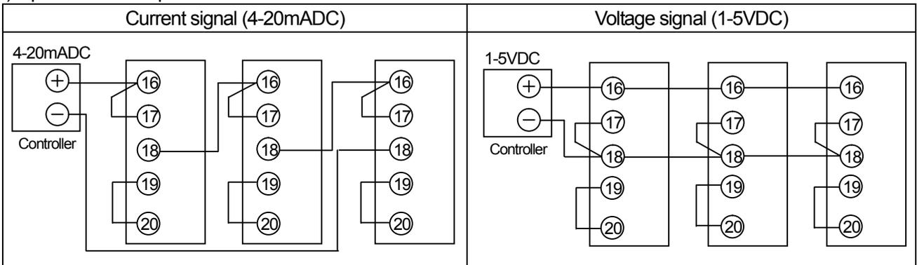
Connectable numbers of the PA-3000-H3 units for plural-unit operation are limited depending on the output capacity of a controller.
