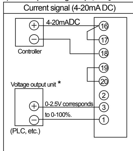
Use the two short circuit plates provided for connections between (16) and (17) (or between 17 and 18), and between (19) and (20), as required. Be sure to check the terminal numbers when connecting them.
