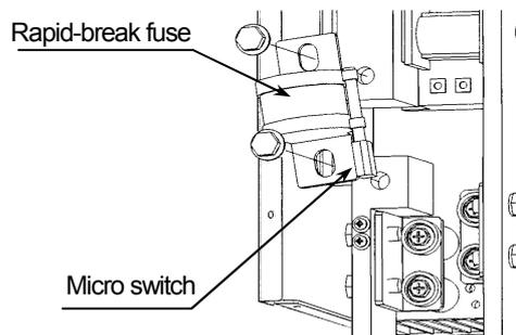
Tightening torque: 25 N·m
