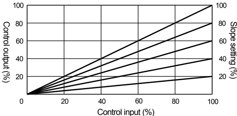
The slope setting provides the output (actually the internal SV used for computational processing) with a slope (inclination). It is effective for example in an electric furnace with 3-zone control where 3 units of the power controller are operated by one controller unit.
