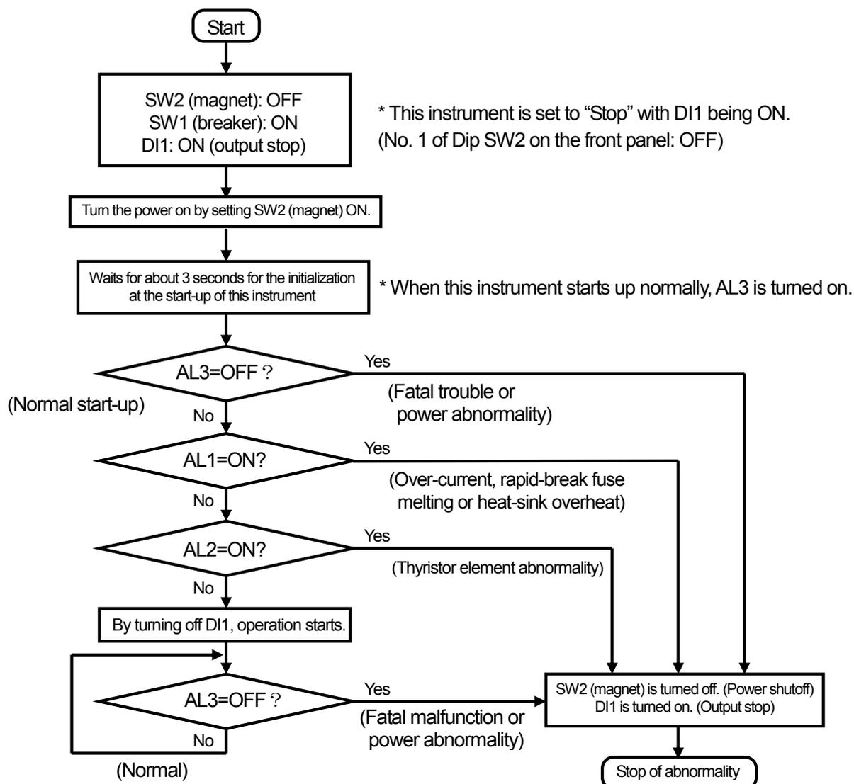
The following is an example of the operation chart when using alarm output 3 (AL3).
