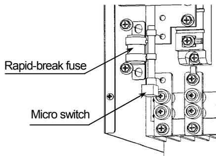
Tightening torque: 3 N·m
