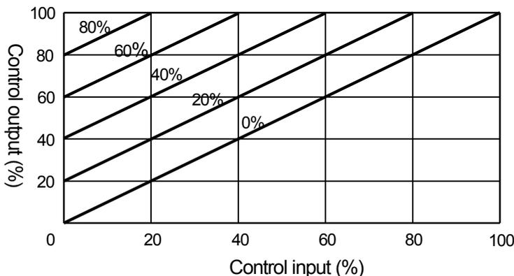
The elevation setting provides the output (actually the internal SV used for computational processing) with a bias. For example, even when the controller output becomes minimum, a constant base power can be applied to an electric furnace, etc.
