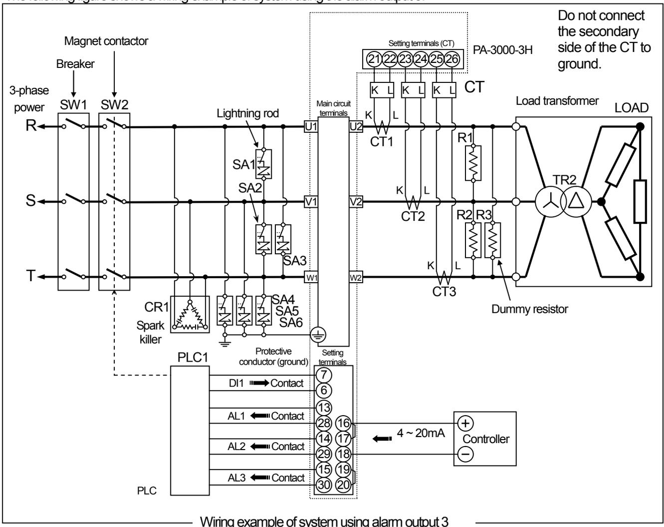
Wiring example of system using alarm output 3
