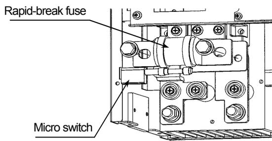
Tightening torque: 12 N·m
