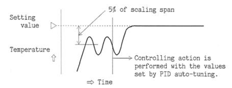
(2) In case of the stable situation during control or when control temperature is within  $\pm 10\%$  of scaling span. Fluctuation is given at the setting value.
