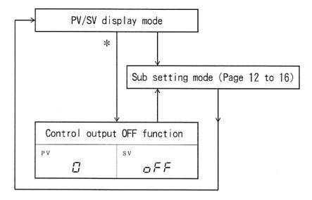
\* In PV/SV display mode, if the (MODE) key is pressed while the  $\blacktriangle$  key is being pressed, the mode turns to Sub setting mode showing the character [P], however, keep pressing until the character [PF] is displayed. (It is for approx. 3s.) To cancel the function, carry out the same key operation.
