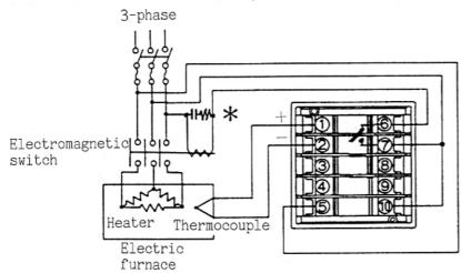
\* To prevent from a bad influence to the instrument owing to the unexpected level noise, it is recommended that the surge absorber be provided between the coil of the electromagnetic relay.
