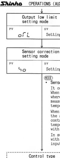
Mode to set the low limit of the control output.
