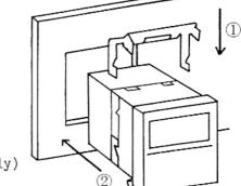
Screw type mounting bracket (Option: BL) (Mounting panel thickness 1 to 8mm)
