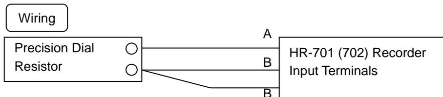
Conduct calibration according to the instructions in 7.2.12 Data Calibration (Calibration of the RTD). (See p.91)
