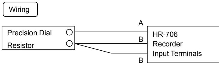
Calibrate RTD according to the instructions in Section “7.2.12 Data Calibration” (Calibration of the RTD). (See pages 83-85.)
