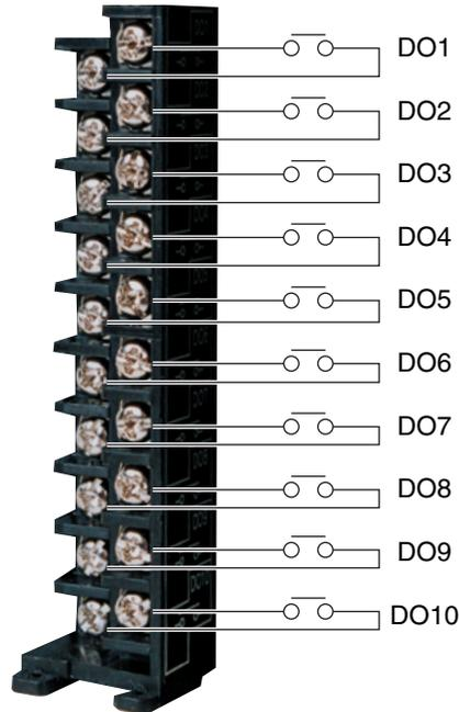
**Note: If lamps are provided on the outside, set a resistor to prevent rush current. When relays or solenoids are used, set elements for contact protection (diodes or surge killers, etc).**
