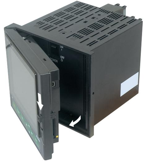
Step 2) Insert the memory card into the slot at the right side of the panel unit as shown in Photo.
