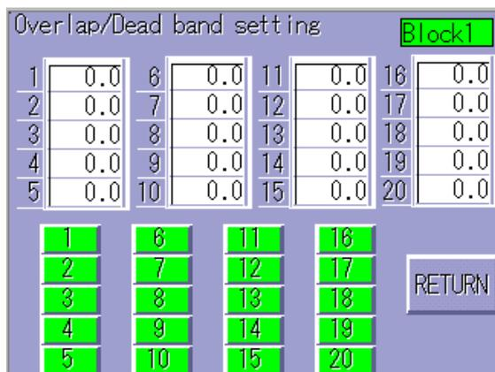
Sets the Overlap band and Dead band for Heating and Cooling control outputs.
