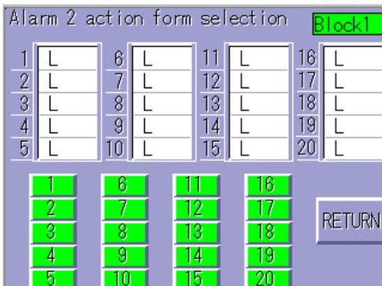
Selects Alarm 2 action form for all channels. Action form: See [Table 5.4-2] above. For alarm action drawing, refer to the instruction manual for the C series.
