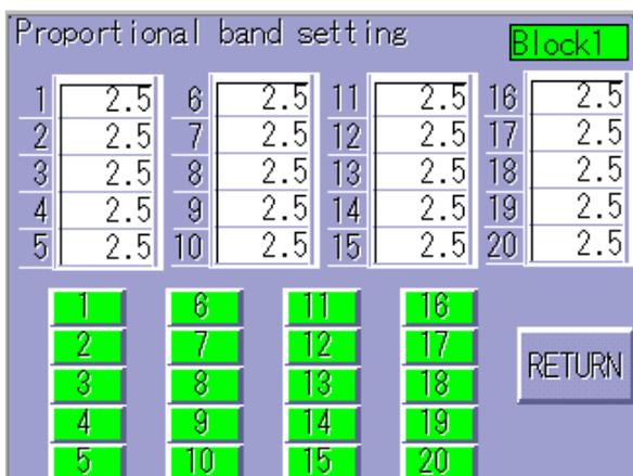
Sets the proportional band for all channels. For details of the proportional band, refer to the instruction manual for the C series.
