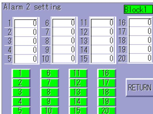
Sets the action point of Alarm 2 output for all channels. However, the setting is not available for the channels that No alarm is selected on the Alarm 2 action form selection display (page 28).
