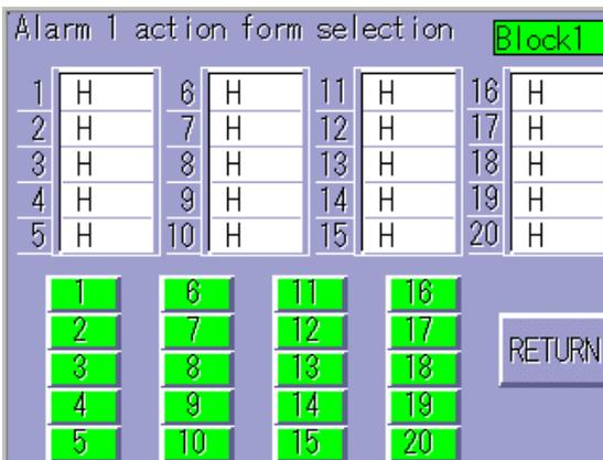
Selects Alarm 1 action form for all channels. Action form: See [Table 5.4-2] below. For alarm action drawing, refer to the instruction manual for the C series.
