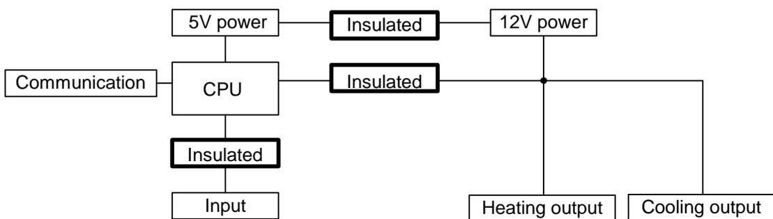
If Heating or Cooling output is relay contact output, Heating output is insulated from Cooling output.
