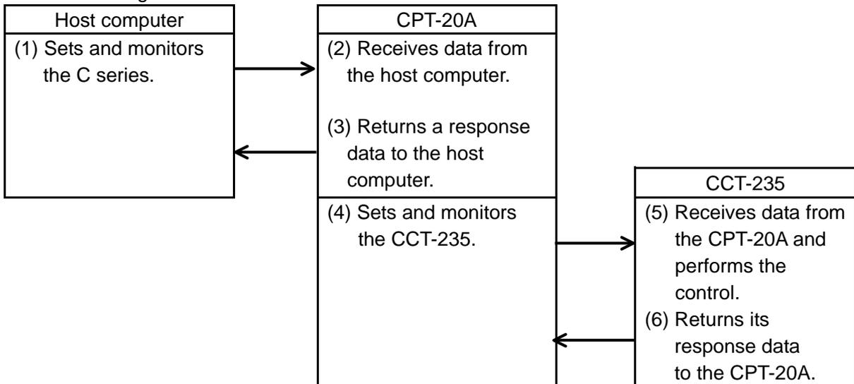
**CPT-20A does not manage the setting ranges of the CCT-235. Therefore, when the host computer sets the set value of the C series, the value should be within the setting range of the CCT-235.**
