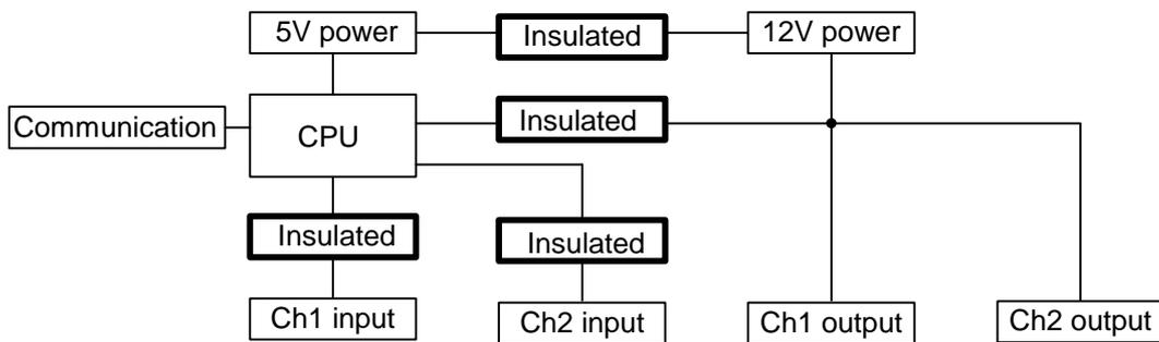
For the relay contact output, Ch1 output is insulated from Ch2 output.
