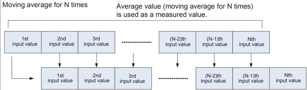
For the next sampling, the 1st input value from the last previous sampling is discarded, and a new input value is added, from which an average value is calculated. This is used as an input value.
