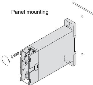
M4 screws can also be used for mounting
