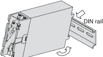
For mounting, hook the unit on the upper side of the DIN rail top to bottom.
