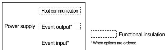
When event input/output is added simultaneously, the connection between event output and power supply is not isolated.
