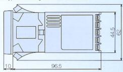
When using screw type mounting bracket (Option : BL)
