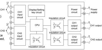
Circuit configuration and terminal arrangement
