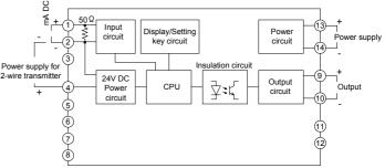
When using as a Current loop supply
