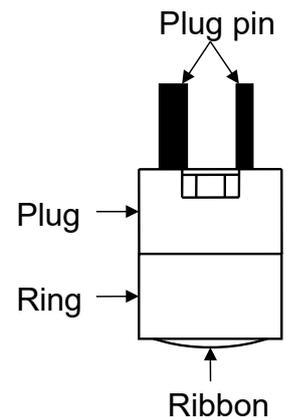
■ **Using the temperature sensor for liquids and the inside of an object: PCE-704, PCE-706, PCE-709, PCR-701**
