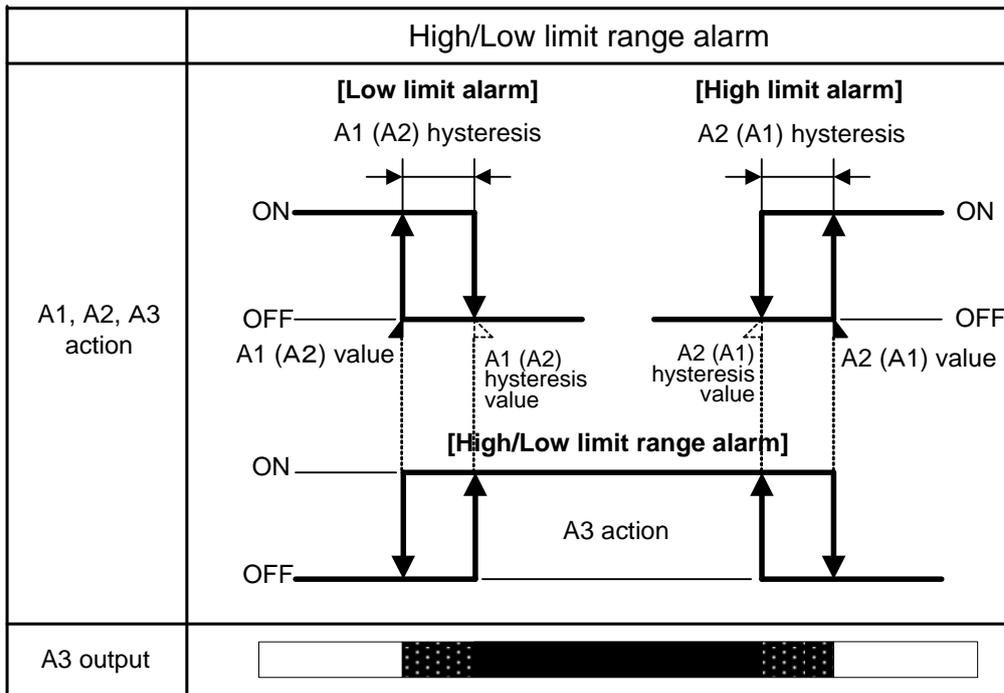
: A1 output terminals (7, 8): OFF, A2 output terminals (9, 10): OFF, A3 output terminals (12, 13): ON
